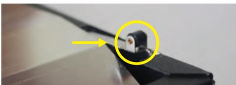
**NOTE:** Deactivating the Snap Switch only shuts off electricity to the UV Light and Fans. The UV Light will be off if you have either disconnected the main power connector or removed the UV Lid to release the Snap Switch. Once the switch is released as you remove the UV chamber cover, the UV lamp will turn off automatically if the unit is still powered on.
